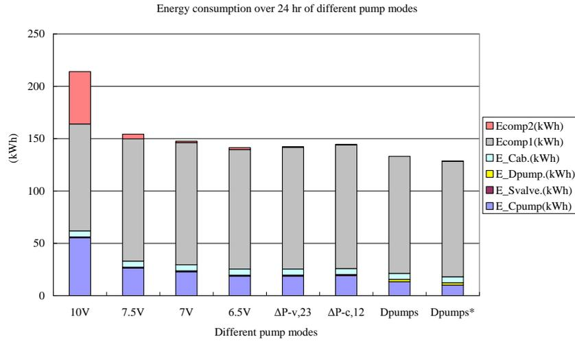
Figure 5. Energy consumption of each equipment over 24 hr for different pump modes.
