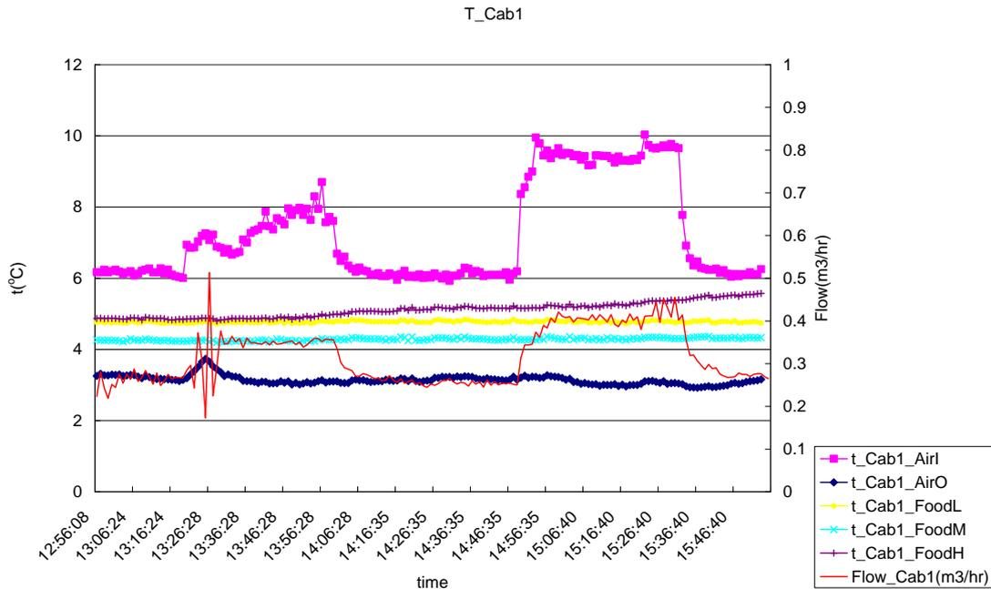
Figure 17 Temperatures and flow curves for Cabinet 1 ( $t_{\text{setting}}=80\%$ ,  $dp\text{-}c=8\text{m}$ ).
