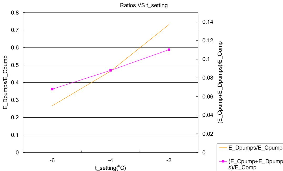
Figure 11 Equipment power ratios VS  $t_{setting}$
