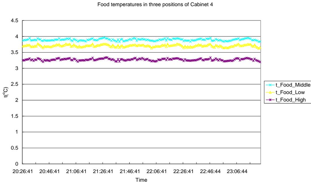
Figure 3-2 Controlled food simulator temperatures in one cabinet.
