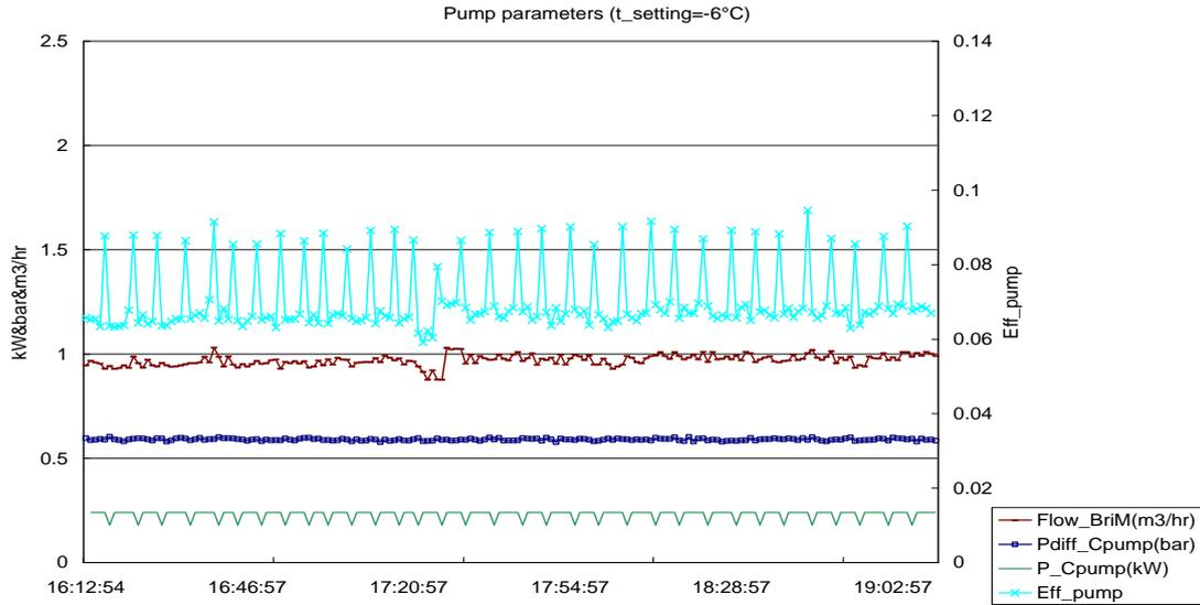
Figure 1 Pump parameters at  $t_{\text{setting}}=-6^{\circ}\text{C}$
