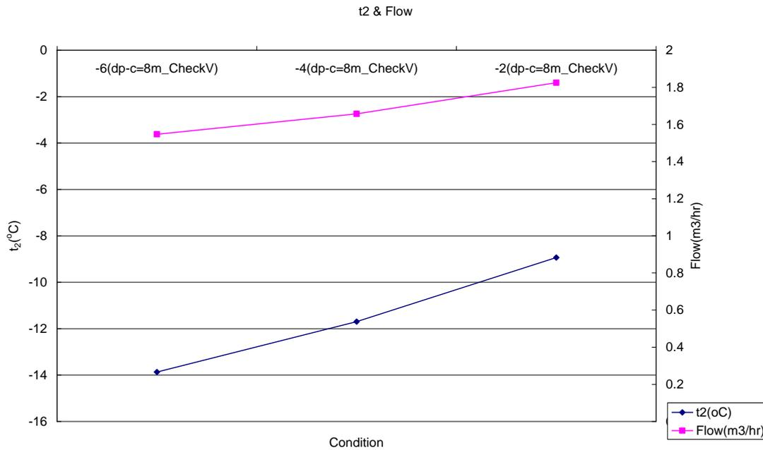
Figure 13 Main brine flow and  $t_2$  in each condition.
