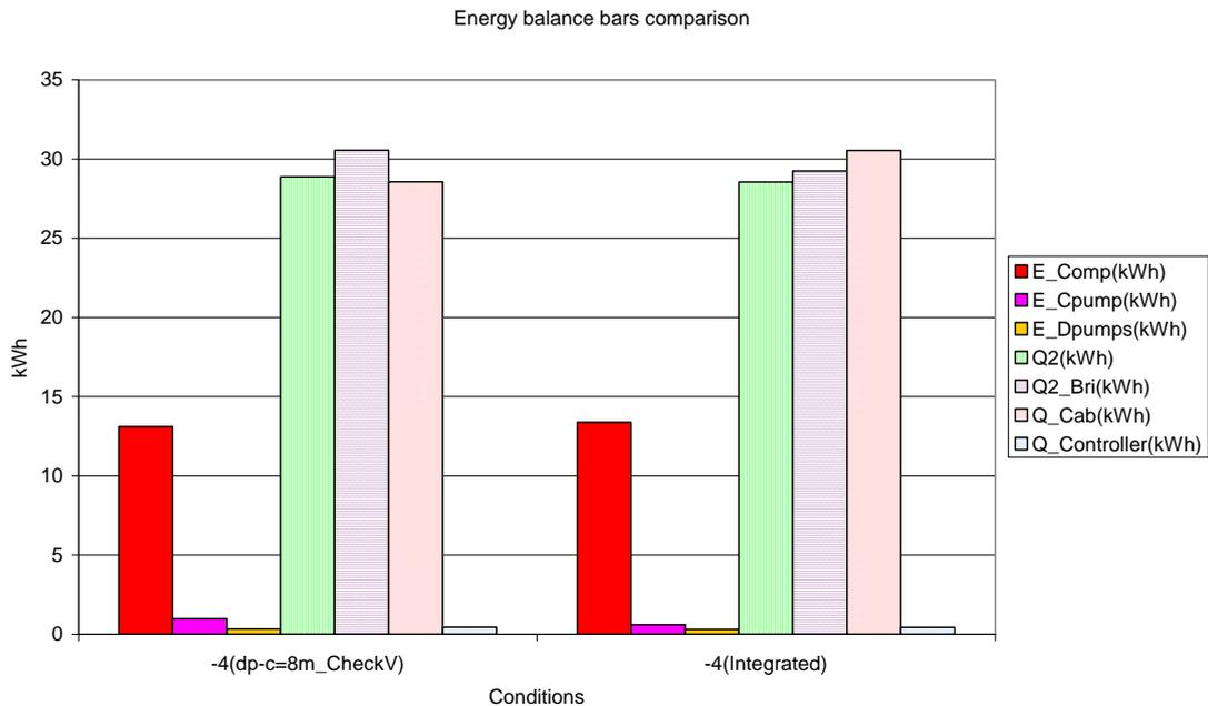
Figure 22 Energy balance comparison between condition  $-4^{\circ}\text{C}$  (dp-c=8m\_CheckV) and  $-4^{\circ}\text{C}$  (integrated control).
