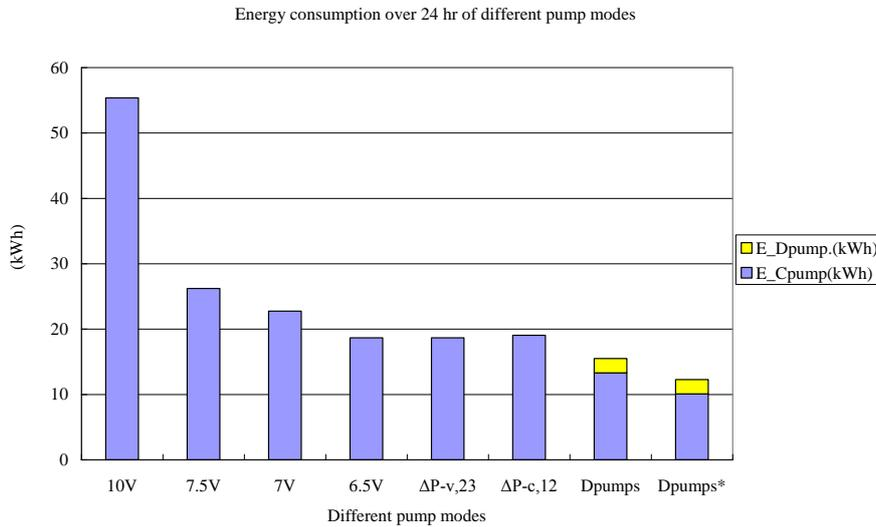
Figure 6. Energy consumption of the pumps only (central and decentralised) over 24 hrs.
