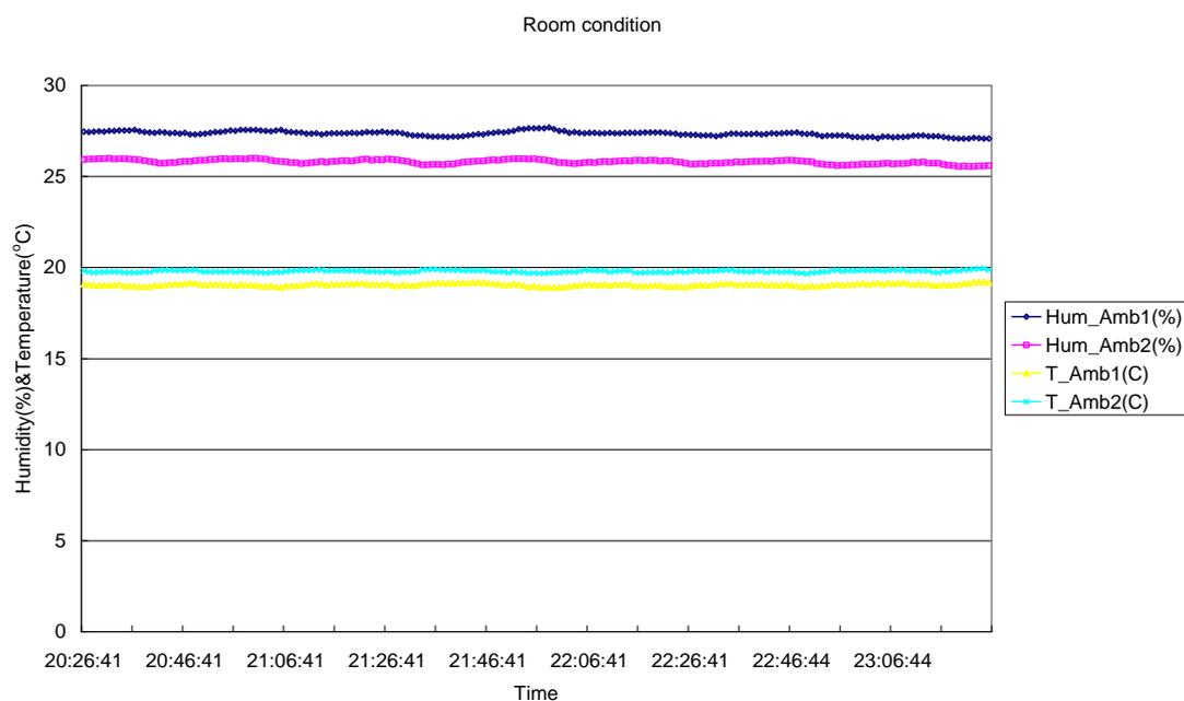
Figure 3-1 Controlled room conditions with temperature and humidity.
