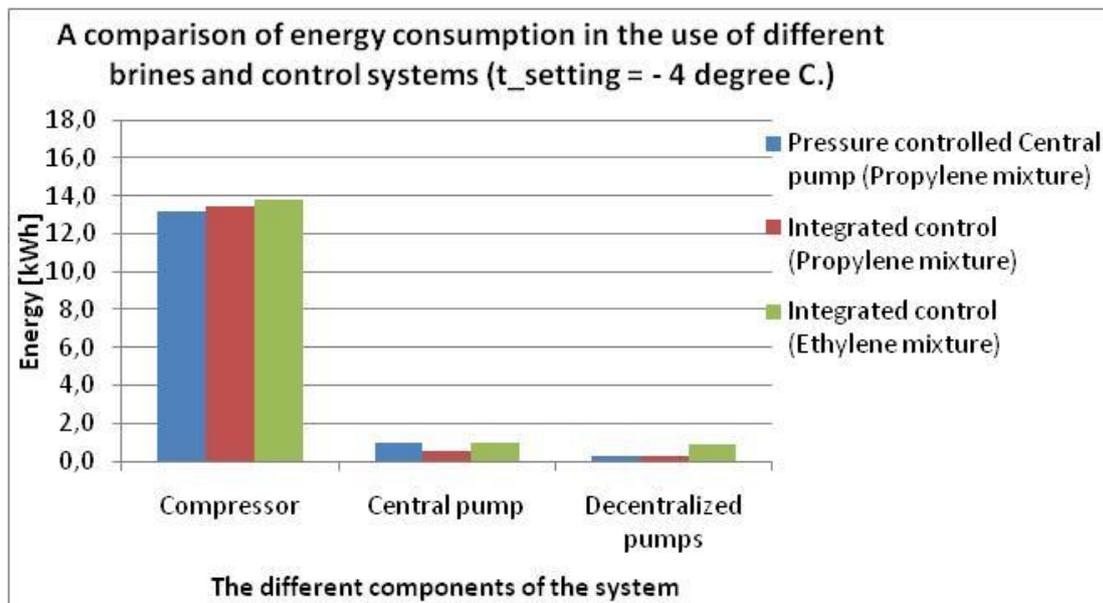
Figure 24 A comparison of energy consumption during three hours for different brines and control modes.
