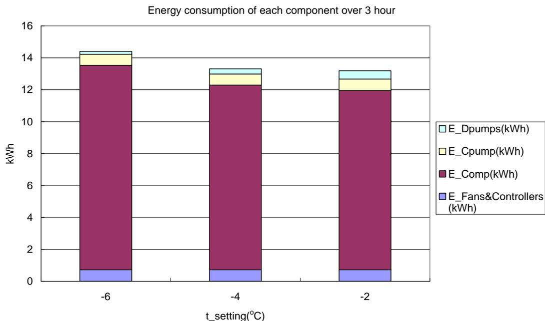
Figure 8 Energy consumption of each component over 3 hours.
