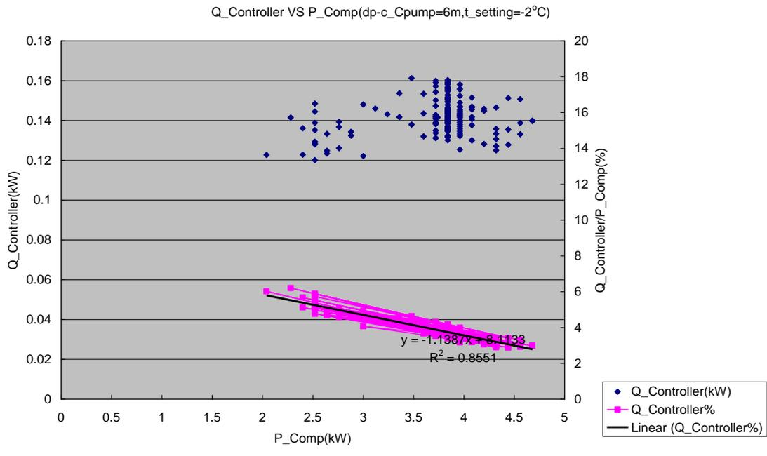
Figure 7 Q\_Controller's real value and proportion VS P\_Comp when t\_setting=-2°C.
