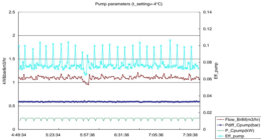
Figure 2 Pump parameters at  $t_{\text{setting}}=-4^{\circ}\text{C}$
