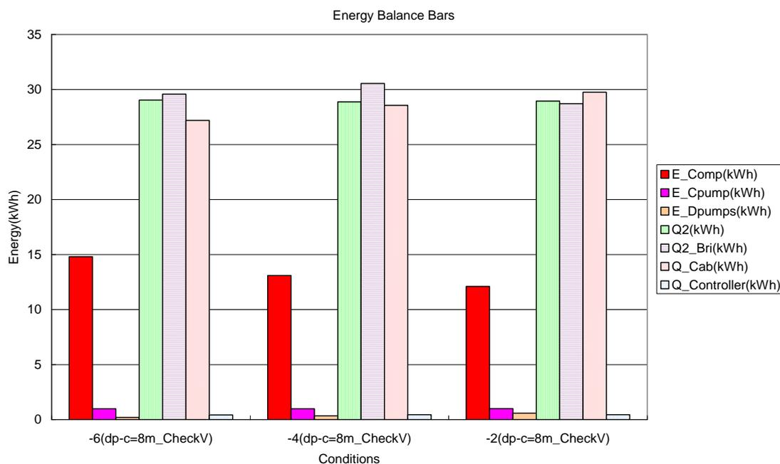
Figure 12 Energy balance bars at  $\Delta p_c=8\text{m}$ .
