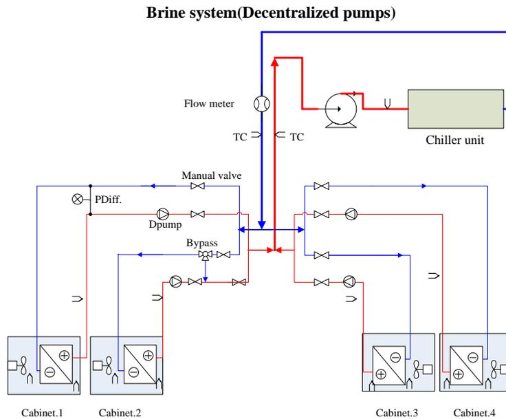
Figure 3. System sketch of the decentralised pump system.
