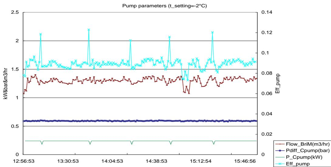
Figure 3 Pump parameters at  $t_{\text{setting}}=-2^{\circ}\text{C}$
