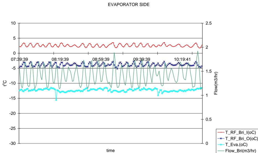
Figure 20 Main brine flow and the temperatures at the evaporator side.
