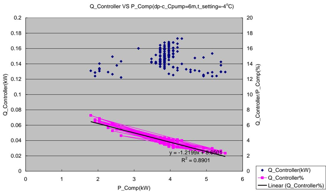
Figure 6 Q\_Controller's real value and proportion VS P\_Comp when t\_setting=-4°C.
