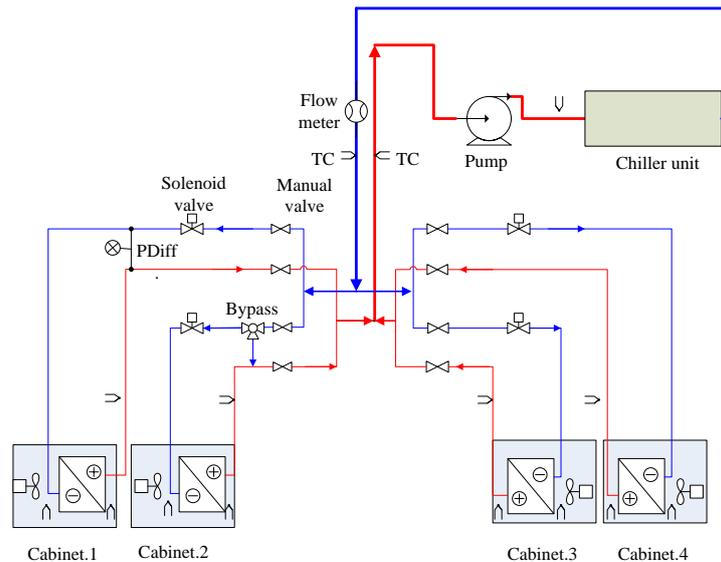
**Figure 2.** The cold side distribution system (secondary loop) of the test system.
