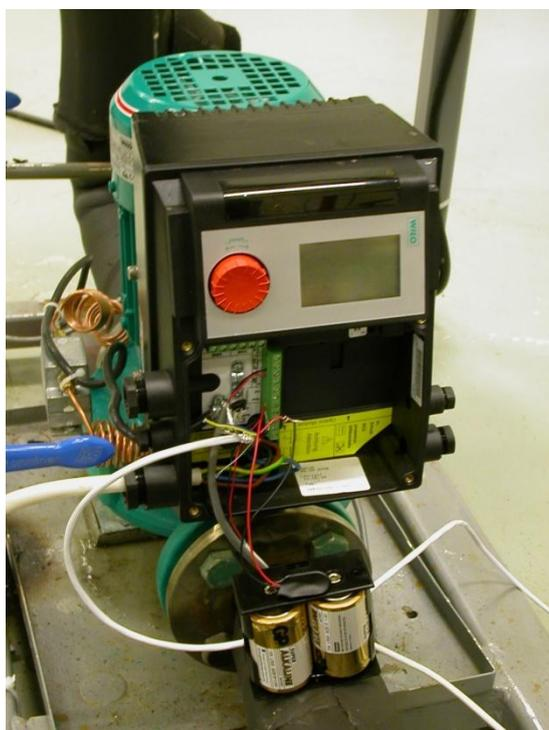
Figure 19 Pump is controlled by the external signal sent from the compressor frequency controller.
