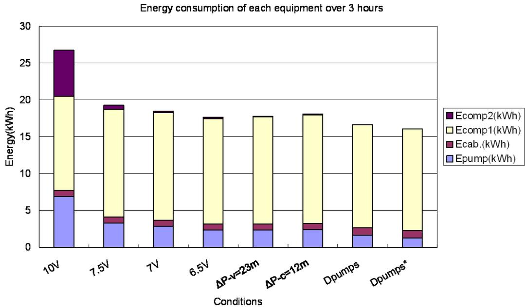
Figure 9 Energy consumption of each component over 3 hours (Phase 1).
