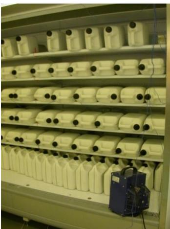
Figure 16 Dynamic heat load change. (high load)
