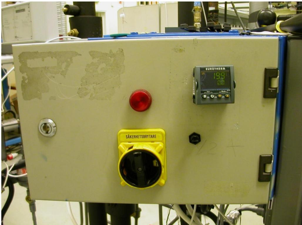
Figure 2-4 Temperature converter for the compressor control.
