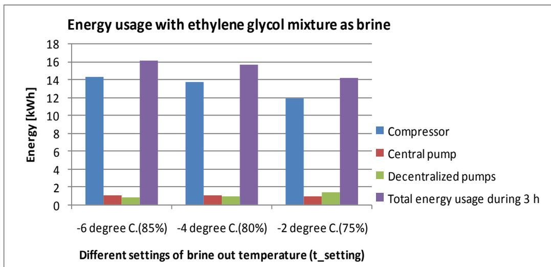
Figure 23 A comparison of energy consumption during three hours for different values of  $t_{\text{setting}}$ .
