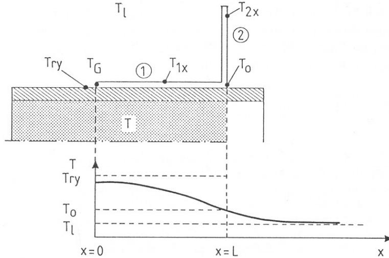
**Figure 7.1** The figure shows the temperature profile along a surface mounted temperature sensor (Fahlén<sup>[16]</sup>).
