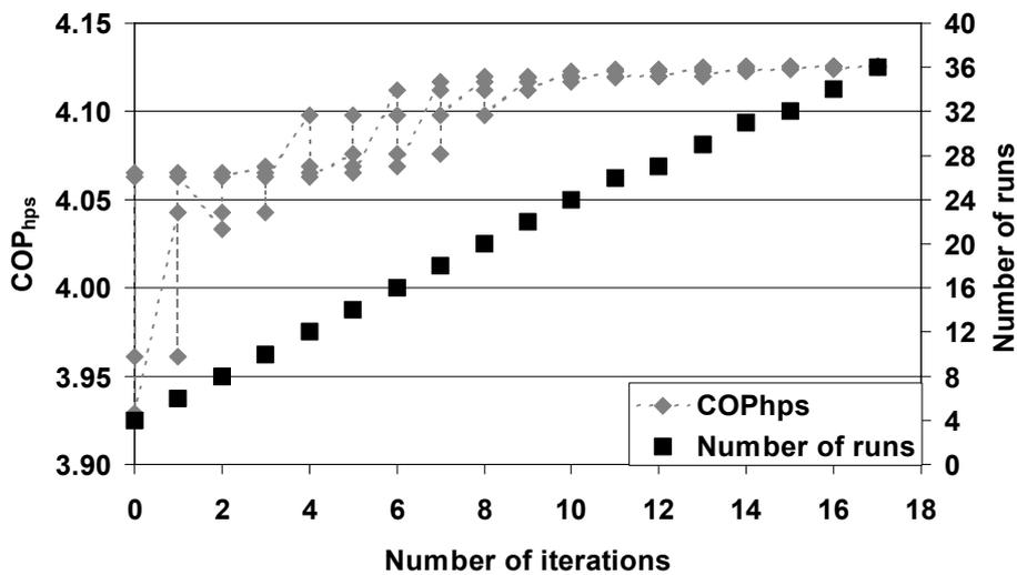
**Figure 5.3** The number of iterations and number of runs (test points) for finding the optimal set-point when  $t_{bi} = -1$  °C and  $t_{wi} = 25$  °C.
