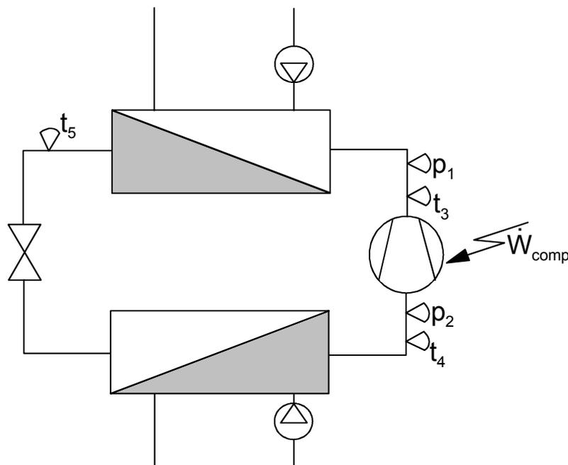
**Figure 4.1** Schematic diagram of a heat pump.
