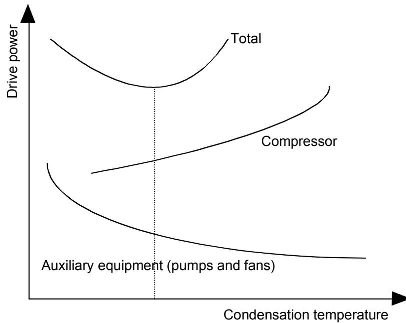
**Figure 2.3** It is possible to find a combination of compressor speed and fan or pump speed such that the total drive power is minimised while the required heating capacity is maintained (Jakobsen and Skovrup<sup>[37]</sup>).
