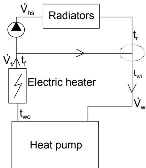
**Figure 6.11** The connection of the heat pump to the heating system. The designations for the different temperatures in the system are also marked.
