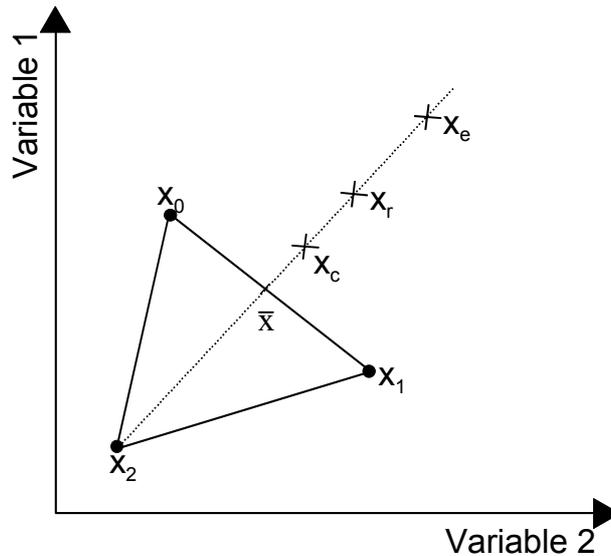
**Figure 4.4** For two variables the simplex forms a triangle. In the picture the three test points and the reflection, expansion and contraction steps are indicated.
