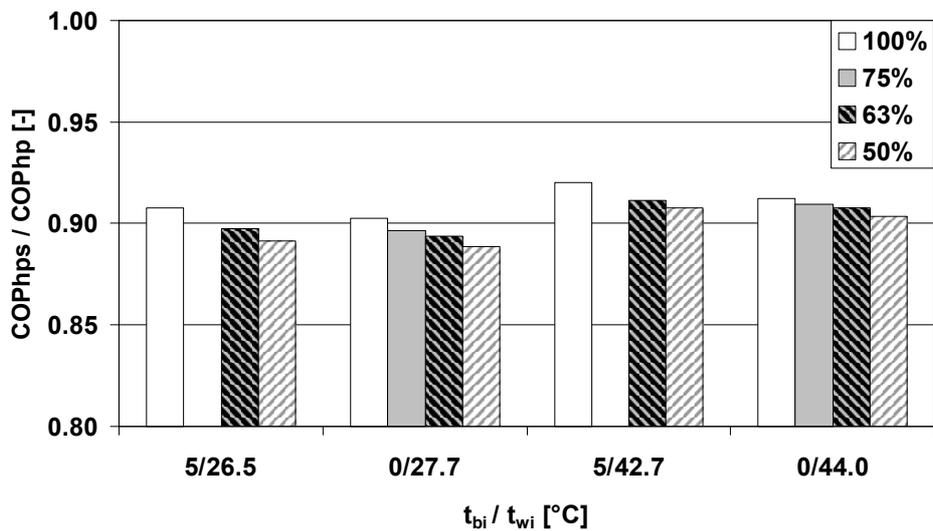
**Figure 6.8** The decrease in coefficient of performance due to the circulation pumps when the compressor is operating on and off. Tests were not performed at the part load 75 % for the operating points 5/26.5 and 5/42.7.
