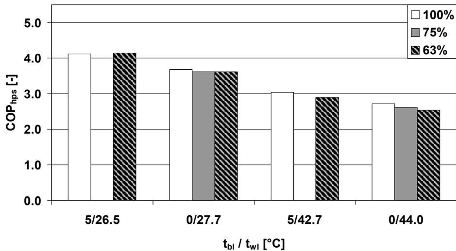
**Figure 6.5** Heat pump system coefficient of performance for variable-speed control (pumps included). The 75 % part load has not been tested for the operating points 5/26.5 and 5/42.7.
