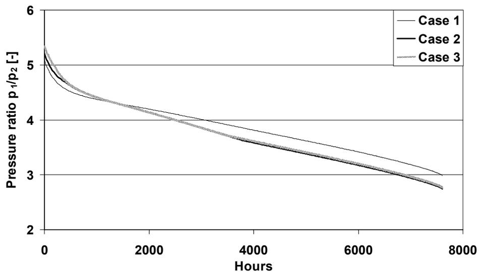
**Figure 6.14** The ratio between condensation and evaporation pressure during the heating season for heat pump size C.
