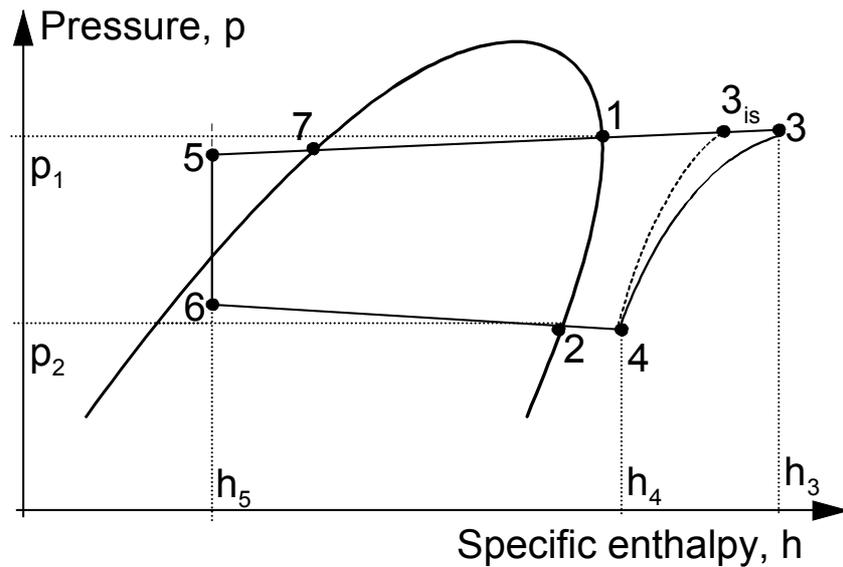
**Figure 4.2** The heat pump process plotted in a Mollier diagram. The numbers correspond to the numbers in Figure 4.1 (Fahlén<sup>[18]</sup>).
