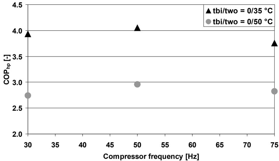
**Figure 6.1** Heat pump coefficient of performance as a function of the compressor frequency for two of the operating points in Table 6.1.
