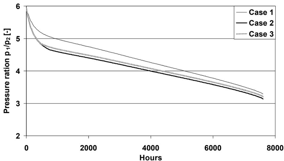
**Figure 6.12** The ratio between condensation and evaporation pressure during the heating season for heat pump size A.
