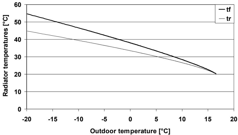
**Figure 6.10** Radiator temperatures as a function of the outdoor temperature for the chosen 55/45 heating system.
