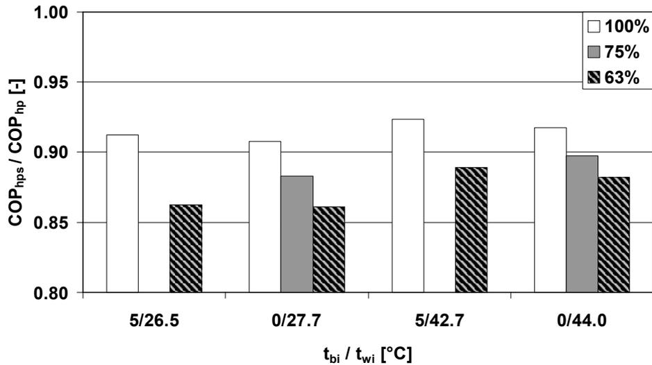
**Figure 6.9** The decrease in coefficient of performance due to the circulation pumps when the compressor is in variable speed operation. Tests were not performed at the part load 75 % for the operating points 5/26.5 and 5/42.7.
