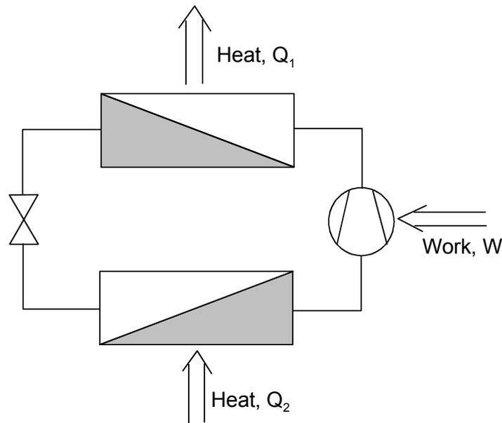
**Figure 1.1** Schematic picture of a heat pump.
