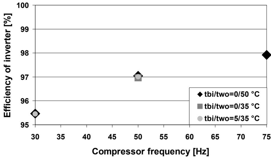
**Figure 6.6** The efficiency of the frequency converter depends on the compressor frequency but not on the operating point.
