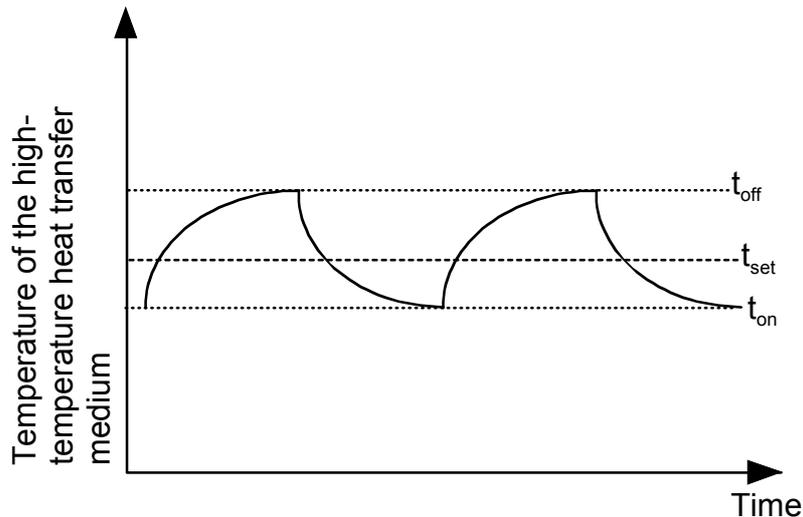
**Figure 2.1** The normal way of controlling a heat pump is to switch it on and off between two limits ( $t_{on}$  and  $t_{off}$ ) in order to keep the desired mean temperature ( $t_{set}$ ).
