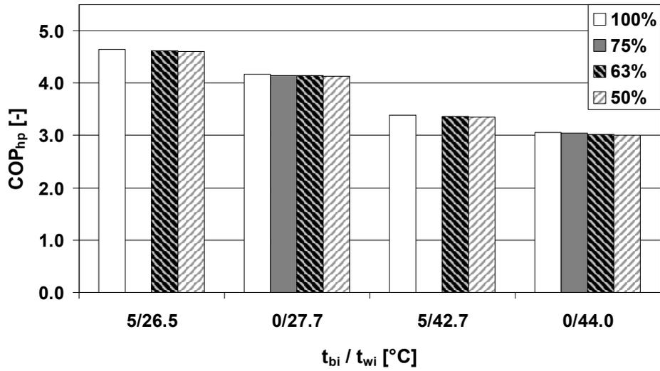
**Figure 6.2** Heat pump coefficient of performance for on/off control (pumps excluded). The 75 % part load has not been tested for the operating points 5/26.5 and 5/42.7.
