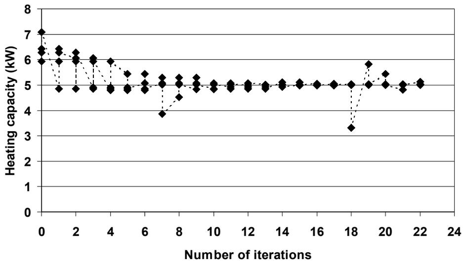
**Figure 5.6** The change of the heating capacity as the optimisation proceeds.
