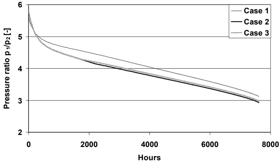
**Figure 6.13** The ratio between condensation and evaporation pressure during the heating season for heat pump size B.
