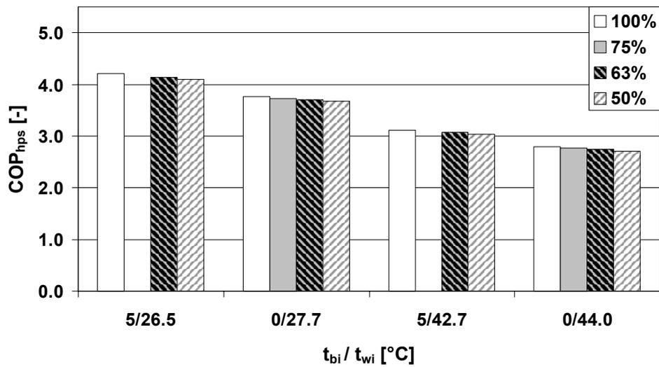
**Figure 6.3** Heat pump system coefficient of performance for on/off control (pumps included). The 75 % part load has not been tested for the operating points 5/26.5 and 5/42.7.
