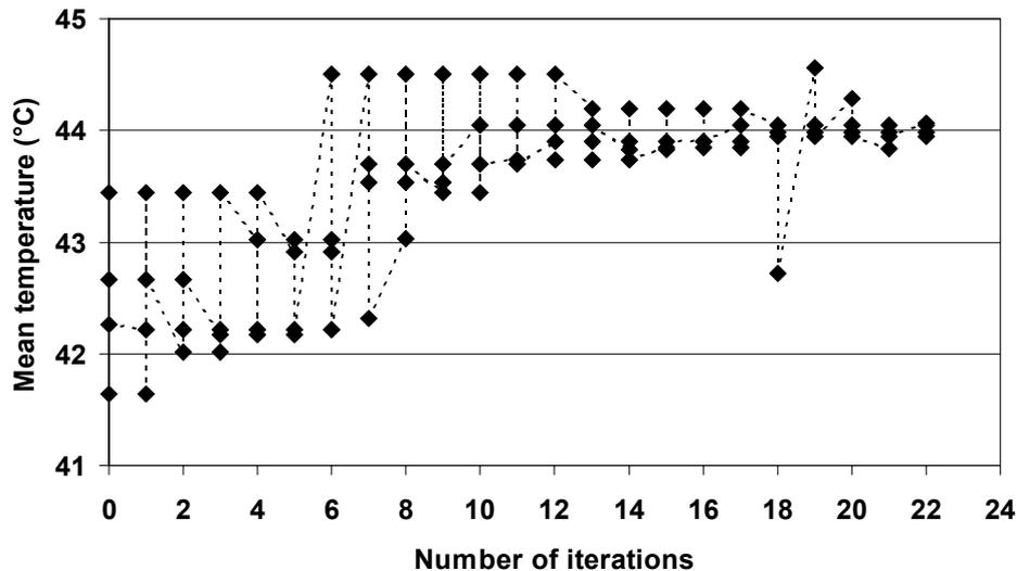
**Figure 5.7** The change of the heating water mean temperature as the optimisation algorithm proceeds.
