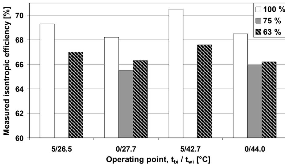
**Figure 6.7** The efficiency of the compressor for different loads and operating points. Tests were not performed at the part load 75 % for the operating points 5/26.5 and 5/42.7.
