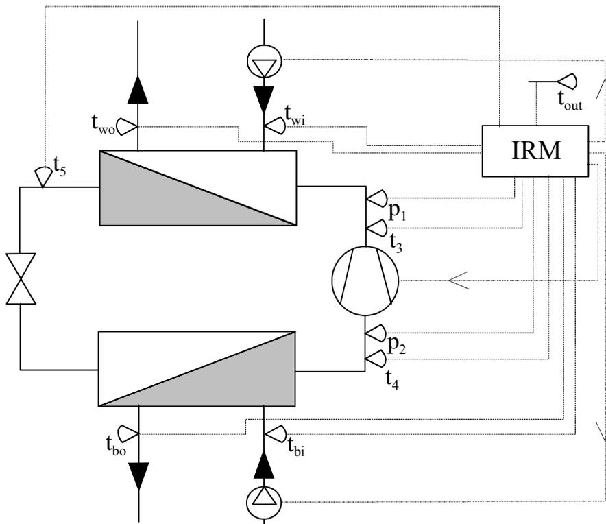
**Figure 7.2** The temperatures and pressures that are normally measured in a heat pump are indicated in this layout. The arrowed dotted lines indicate the signals sent to the controlled components.
