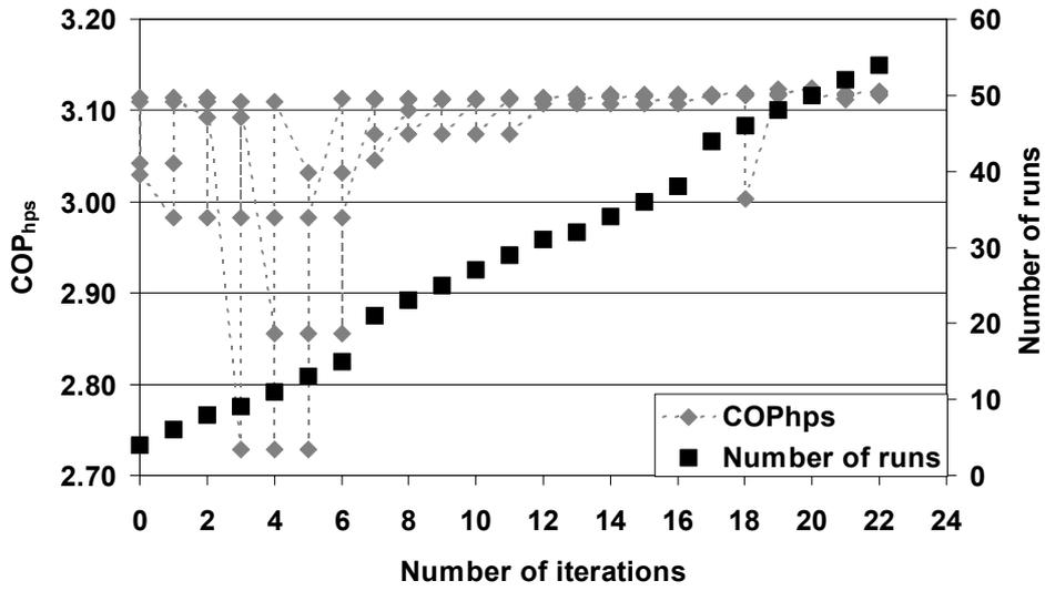
**Figure 5.5** The value of the coefficient of performance and the number of runs necessary to reach the optimal set-point.
