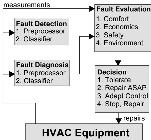
**Figure 2.4** The different steps in fault detection and diagnosis (Rossi and Braun<sup>[60]</sup>).
