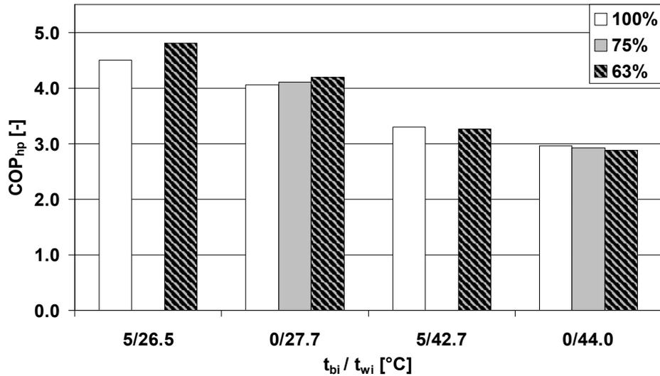
**Figure 6.4** Heat pump coefficient of performance for variable-speed control (pumps excluded). The 75 % part load has not been tested for the operating points 5/26.5 and 5/42.7.
