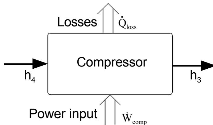
**Figure 4.3** Energy balance for the compressor (Fahlén<sup>[18]</sup>).
