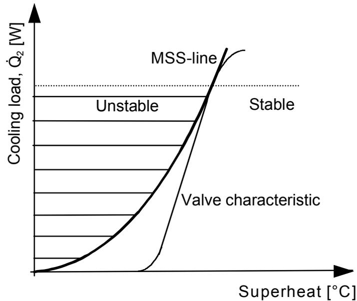
**Figure 2.2** The MSS-line illustrates the limit for stable superheat control.
