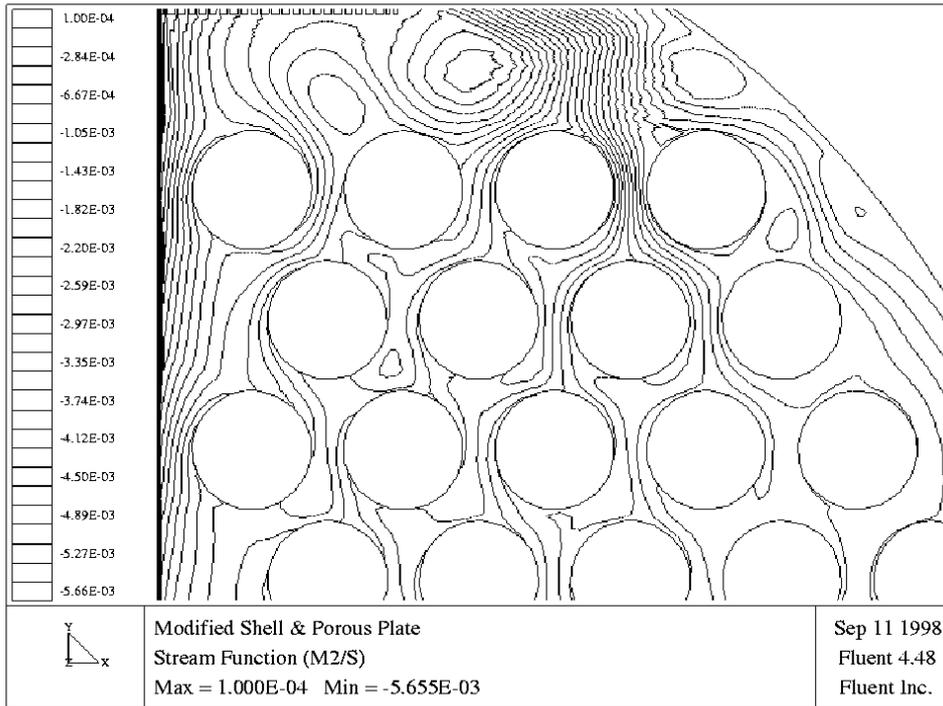
**Figure 7:** Streamlines for the case with decreased shell-side by-pass porous plate.
