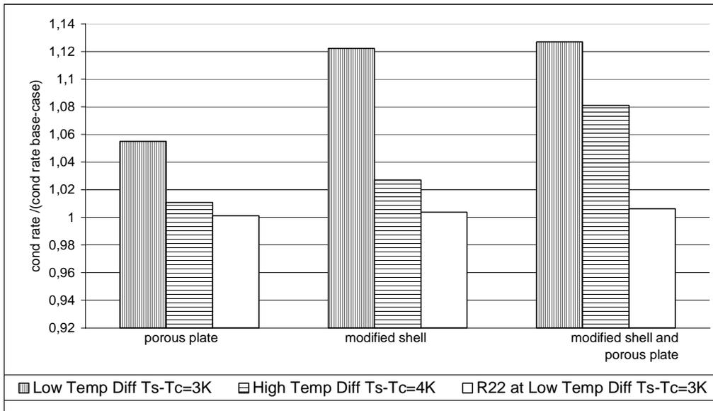
**Figure 4:** Change in the condenser performance for different geometrical modifications.
