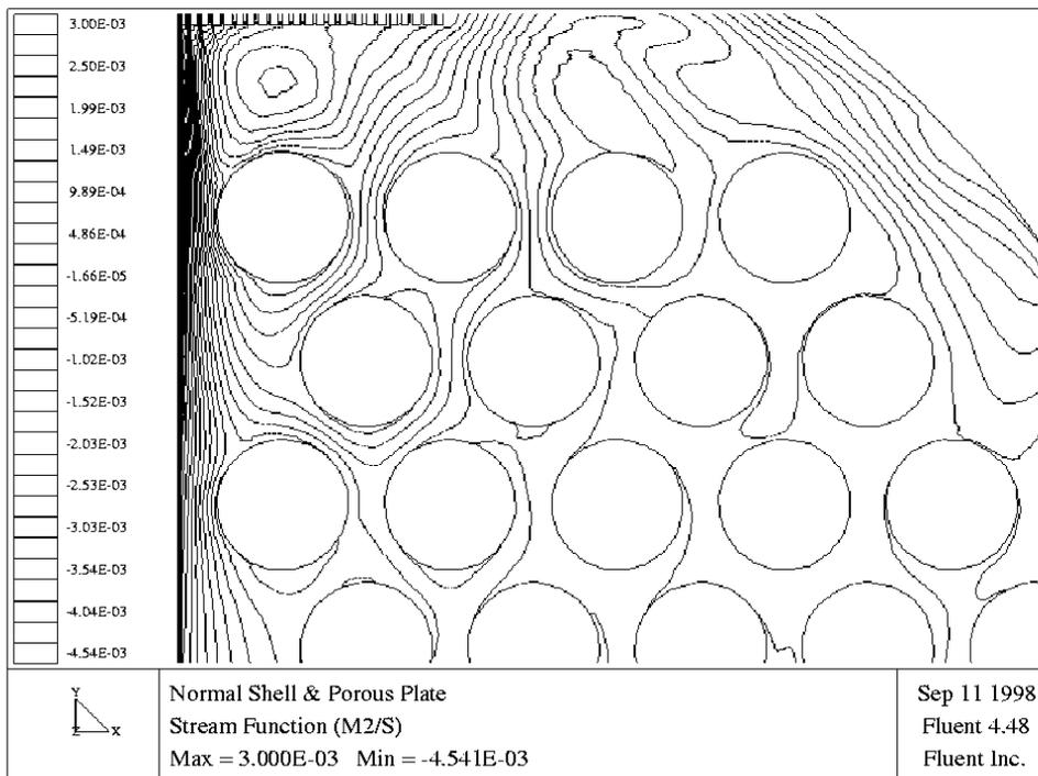
**Figure 6:** Streamlines in case of the porous plate.
