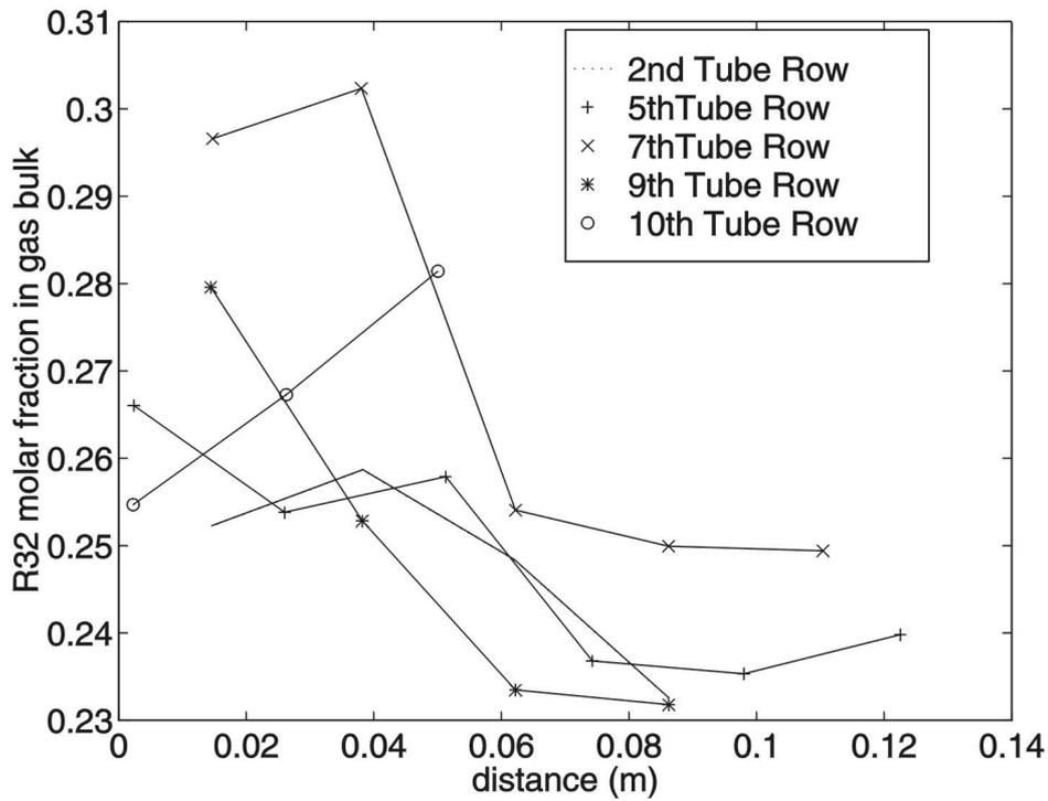
**Figure 8:** Variation of R32 molar fraction along tube length for “base-case geometry” (starting from the symmetry line in Fig. 1).
