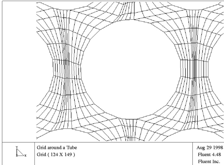
**Figure 2:** Computational grid around a tube.
