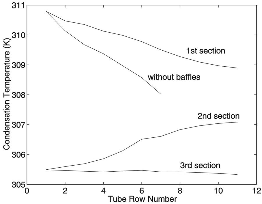
**Figure 3:** Variation of the condensation temperature for single shell and for the same shell with three baffle sections.
