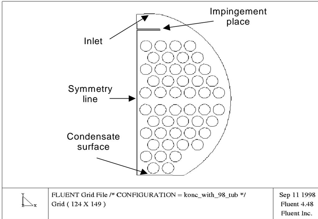
**Figure 1:** Condenser geometry.
