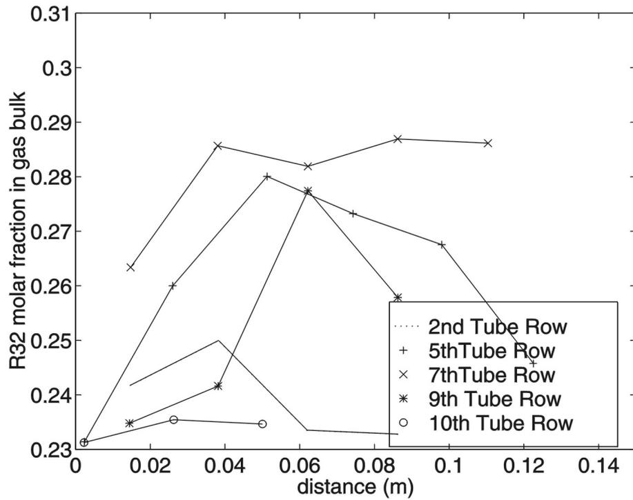
**Figure 9:** Variation of R32 molar fraction along tube-length for the case with decreased shell-side by-pass.
