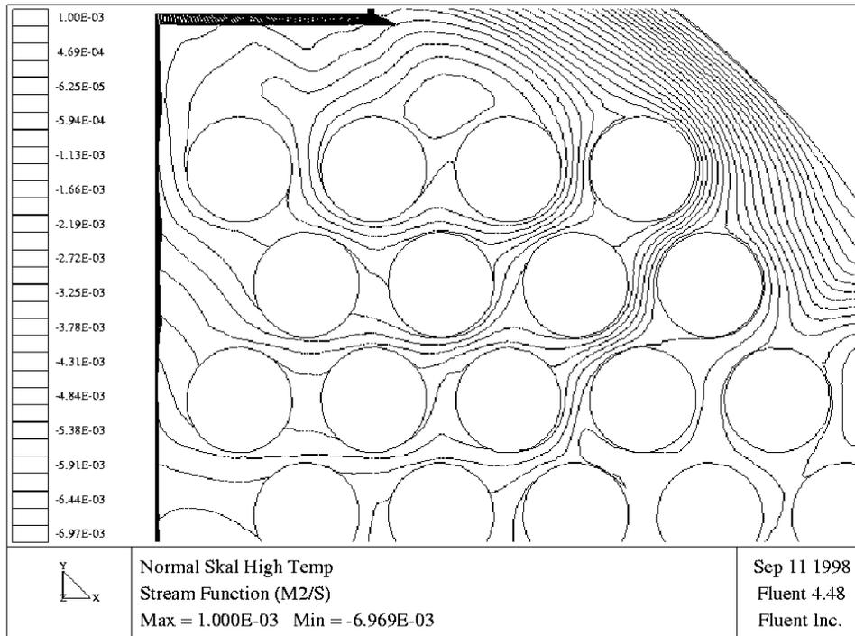
**Figure 5:** Streamlines for the "base-case geometry" at higher coolant to gas temperature difference.
