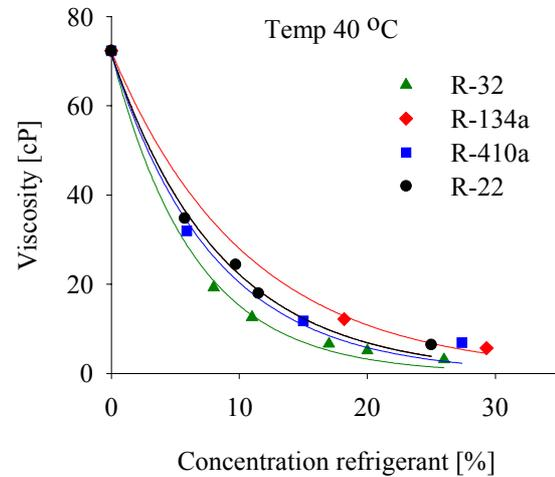
Figure 2 Viscosity vs. concentration 40°C.
