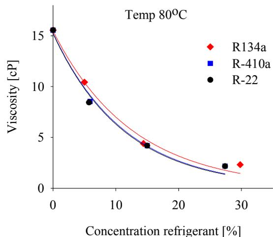
Figure 3 Viscosity vs. concentration at 80°C.
