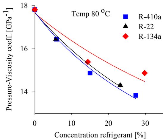
Figur 5 Pressure-Viscosity coefficient vs. concentration at 80°C.
