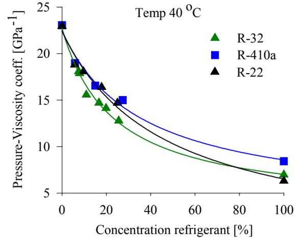
Figure 6 Predicted pressure-viscosity coefficient vs. concentration.
