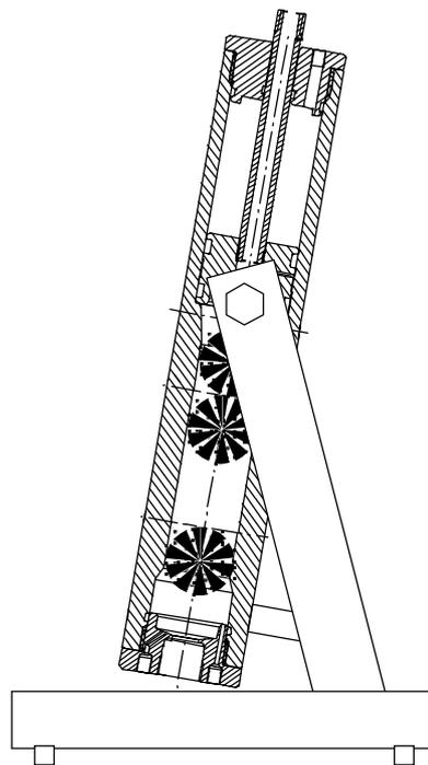
Figure 1 The modified Höppler viscometer.
